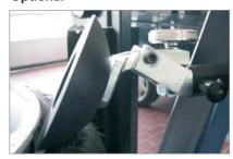
The plastic bead breaker disc is a useful accessory to prevent any damage to the rim
