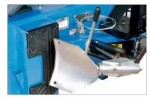
Special bead breaker blade to protect tyre and rim
