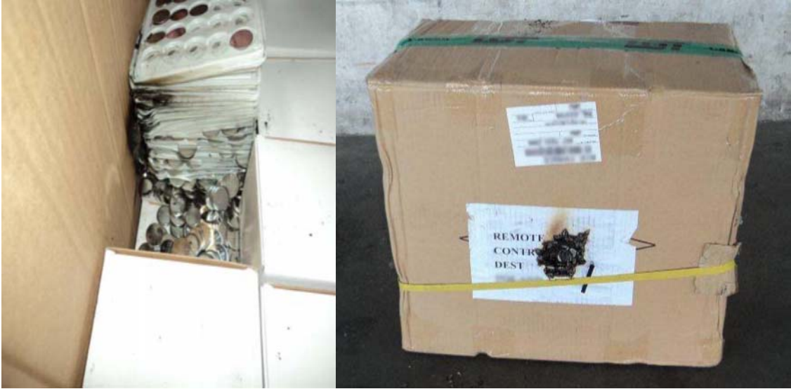
Figure 2 – Short circuit and the resulting fire damage of an undeclared package of lithium metal button cells
