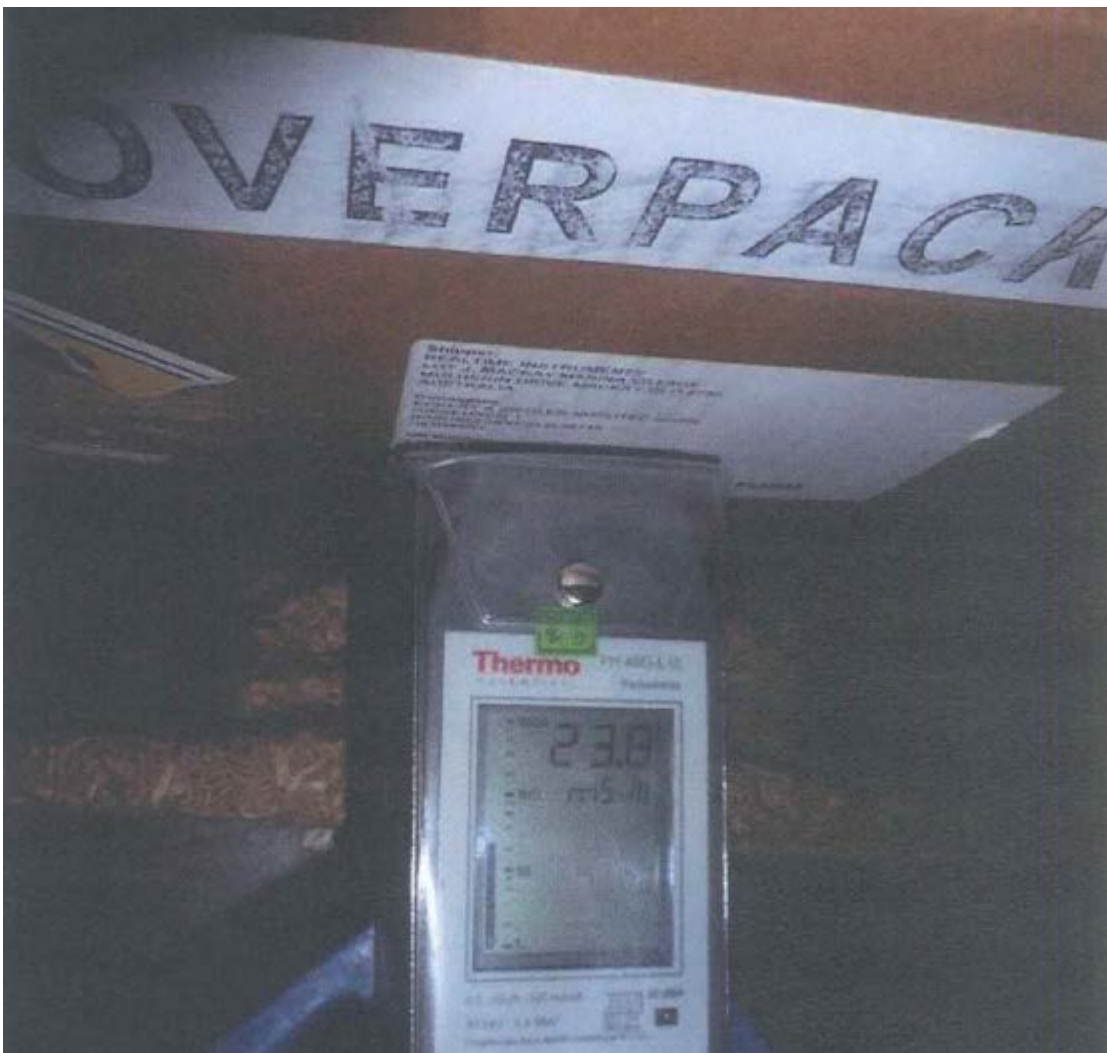
Surface level reading of 23.8 mSv/h on arrival at Frankfurt Airport
