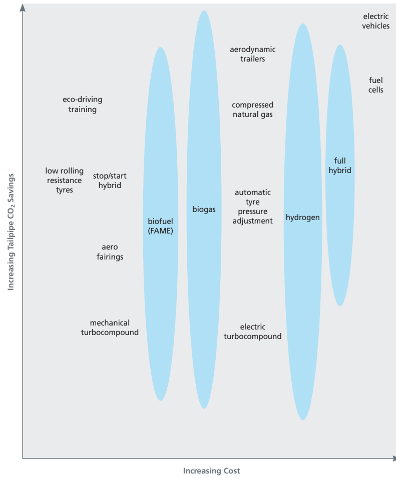
FIGURE 11 Relative Cost-effectiveness of Low Carbon Truck Technologies and Practices (Adapted from Ricardo / UK Department for Transport) 31
